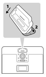
• To remove the adapter, hold its left and right sides and gently pull it up.
